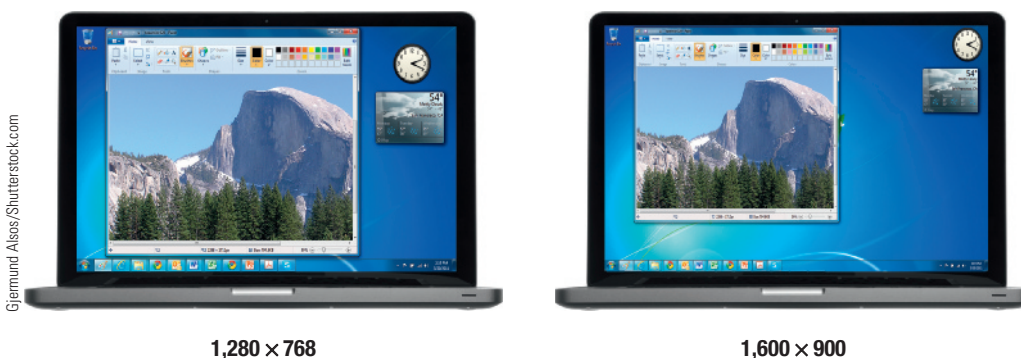
FIGURE 4-27 Screen resolution. A higher screen resolution (measured in pixels) displays more content than a lower screen resolution, but everything is displayed smaller.
