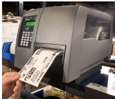
BARCODE PRINTERS Used to print barcoded labels. Some printers can also program RFID tags when they are embedded inside the barcoded labels.
