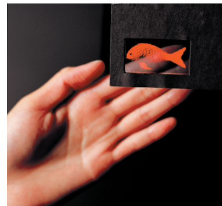
TOLEDs Used to create transparent displays.
