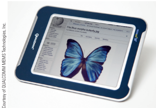
FIGURE 4-33 An IMOD display is bright and readable, even in direct sunlight.
