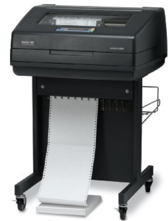
FIGURE 4-35 Dot-matrix printers. Dot-matrix printers are impact printers; today they are typically high-speed printers used in manufacturing, shipping, or similar applications.
