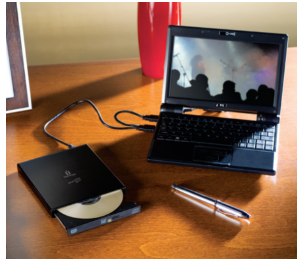
FIGURE 3-12 External optical drives. Can be connected as needed, typically via a USB port, such as to the netbook shown here.
