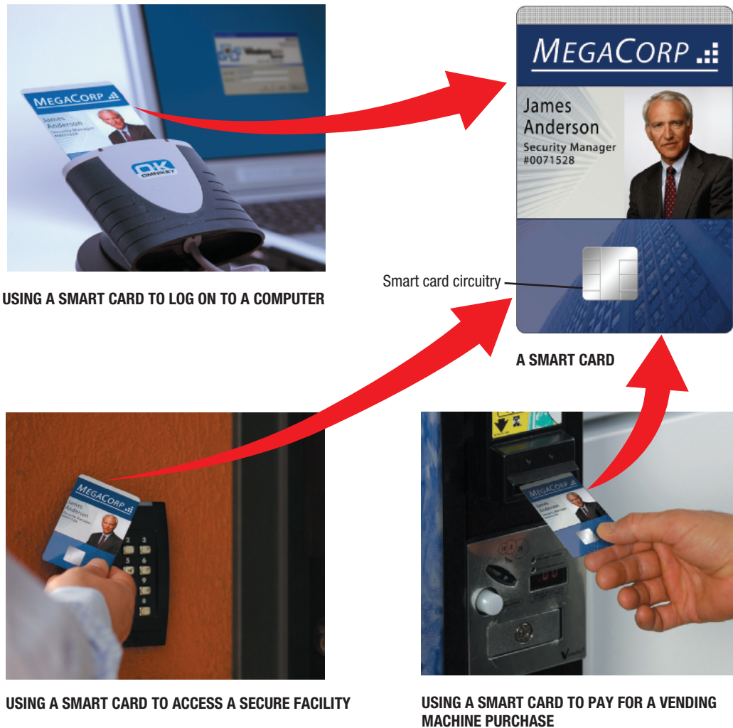
FIGURE 3-21 Smart cards. Smart cards can be used to log on to computers and networks, access facilities, pay for goods and services, and so forth.
