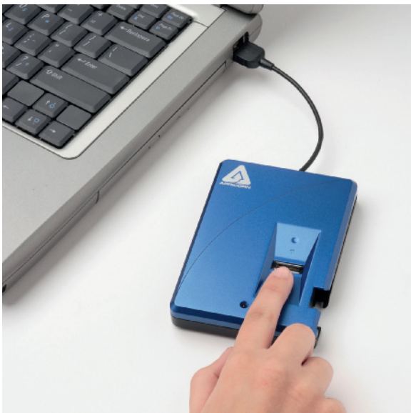
FIGURE 3-3 Encrypted hard drives. The data stored on this external hard drive is protected by a fingerprint scanner.
